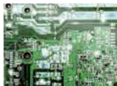
Special coating prevents any damages from humidity and insects.
